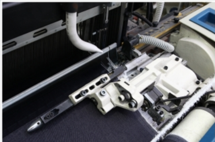
适合重磅织物的幅撑结构 Temple for heavy fabric
